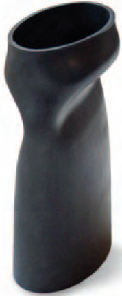
EHS stub column after failure, by inelastic local buckling or “squashing”; this mode of failure resembles plate buckling more than cylinder (shell) buckling.
